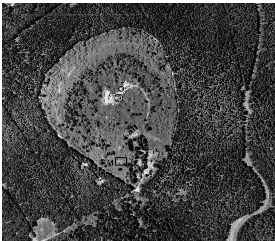
Figure 8.7: Aerial photo of the Taunus Observatory. The large circle shows the measurement site for the peroxy radical and other measurements for the period 1996-99. The \text{RO}_x measurements in 1995 were made in a container marked by the smaller circle at the top. The meteorological garden, where most of the measurements of the DWD were made is marked by a square and the letter M. The wind measurements of the DWD were made on a mast slightly to the right of the large circle.
