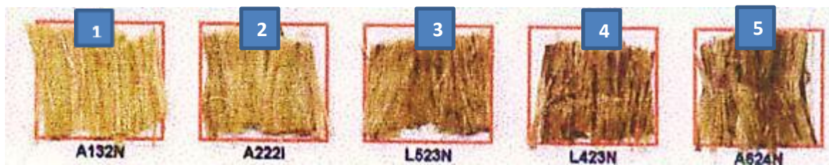
Figure 65. Hemp fibre colour chart used to conduct subjective assessment of retting degree [Source : Own development] .
