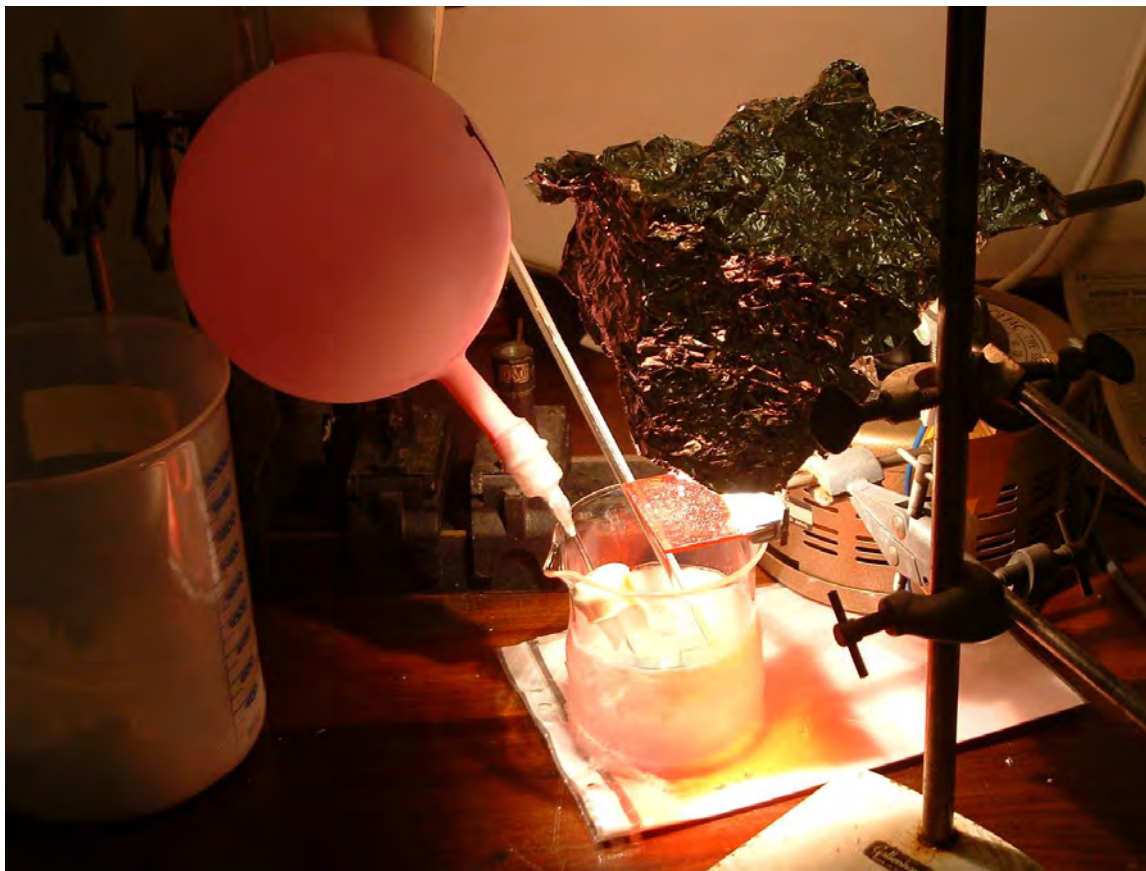
Figure 3.3: Apparatus used in the photooxidative bipyrrrole coupling reaction.
