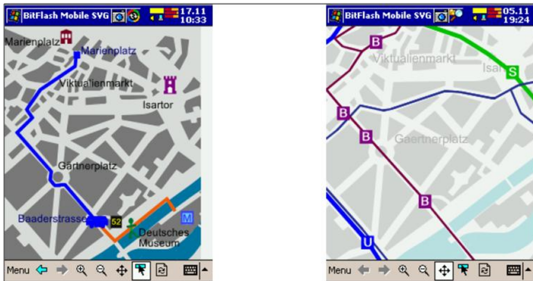
Figure 3.11: Presentation adaptation in an MMV system. The visualisation of a planned route is adapted according to the whether the user is walking (left) or taking a bus (right) (Reichenbacher 2004)
