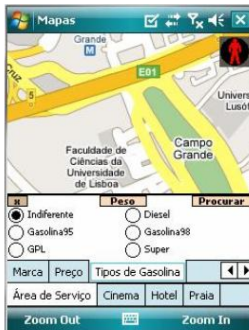
Figure 3.9: An example of interface adaptation in an MMV system. Tabs are ordered based on previous user behaviour (Carmo et al. 2008)
