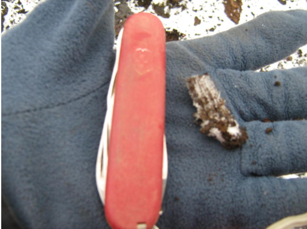
Figure 10: Needle ice with sediment inclusion measured within the disturbed areas around the logger on the morning of 4 December 2008 (9cm knife is used as length of reference).
