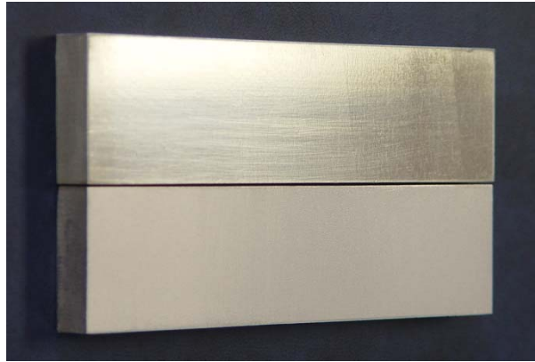
Figure 3.1: Surface reflectivity before and after wire brushing. Original test sample at the top, wire brushed sample below.
