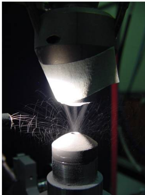
Figure 3.22: Visual inspection of the alignment between the coaxial nozzle work axis and the alignment test jig work axis (centre of the conical nozzle) representing the beam propagation axis
