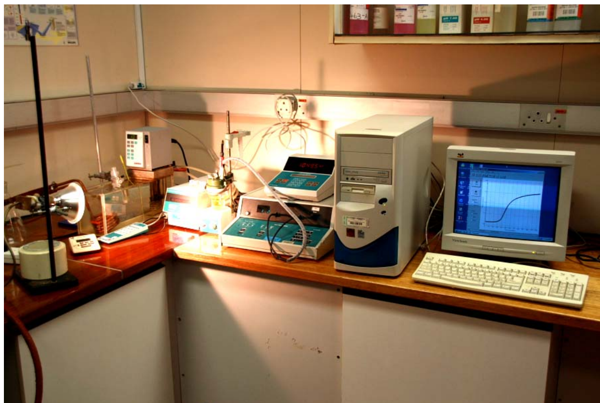
Figure 2.1: Picture illustrates the experimental system employed to record kinetic data during a photosensitive reduction.
