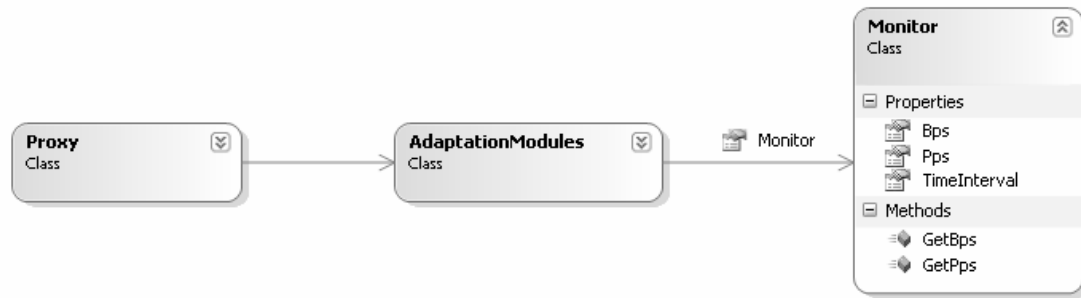
Figure 4-7. System architecture of the responsive content adaptation approach.
