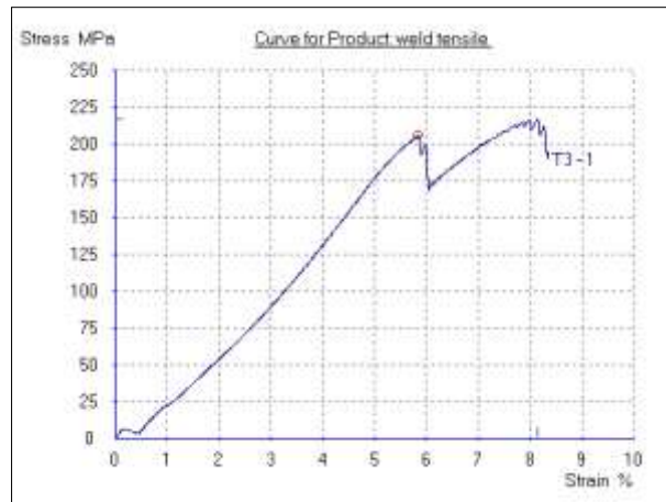
Figure 0.5 Tensile Test data – 140mm from plunge (start) position (UTS 216 Mpa)
