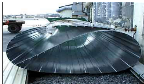
Figure 0.15 Prefabricated FSW panel for catamaran side-wall, rolled for road transport (at Hydro Marine Aluminum) [22]
