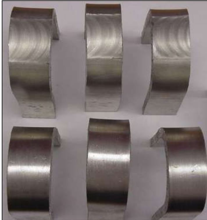
Successive Face (top) and Root (bottom) 180 0 bend tests perform on a weld made at 400rpm, 0.2 Plunge and 100mm/min.
