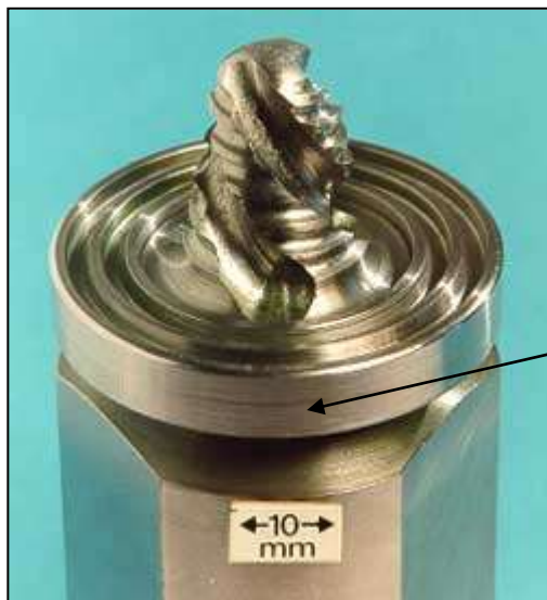
Figure 4.1. In tool as shown in the shoulder and a probe.
