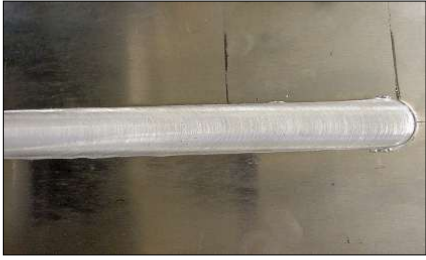
Figure 0.23 Figure illustrating the good surface finish with no surface defects. Weld was made to evaluate the regression formula reliability.
