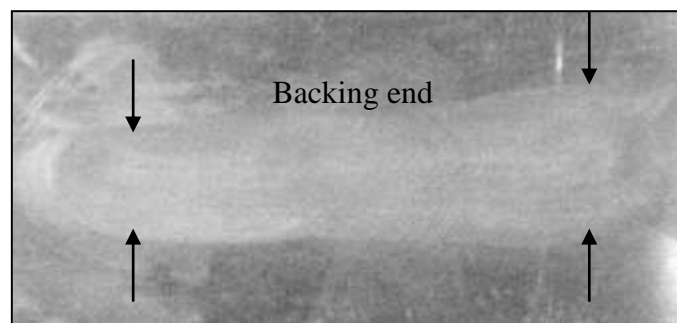
Figure 0.7 Increase in surface rubbing velocity causing incomplete temperature distribution and a decreasing heat pattern (Aluminum 650rpm @ 60mm/min)
