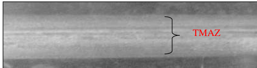
Figure 0.5 Figure illustrating the complete penetration of the heat throughout the plate viewing it from the backing end (Alluminum - 400rpm @ 60mm/min)
