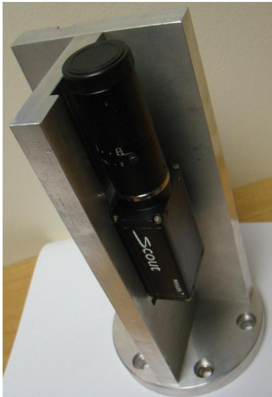
Figure 5.6: Manufactured Bracket with the Camera Mounted Thereon
