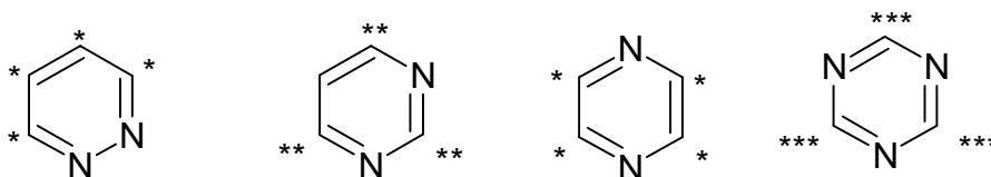
Figure 1.11 The selective activation of ring carbon atoms (asterisks indicate the number of ortho or para nitrogen atoms) 19
