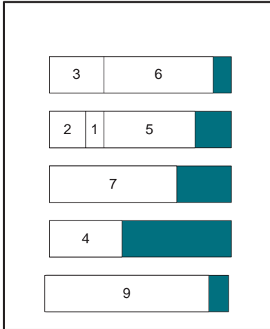
Figure 4.1: A possible solution for one dimensional bin packing problem, where the shaded areas represent waste.
