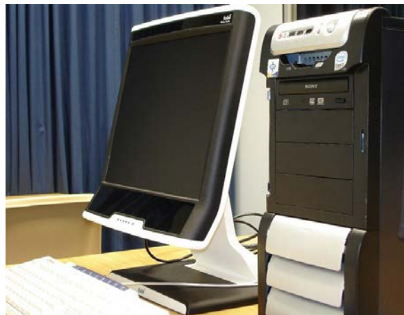
Figure 7: The Tobii T60 eye tracker (usability laboratory - participant room)
