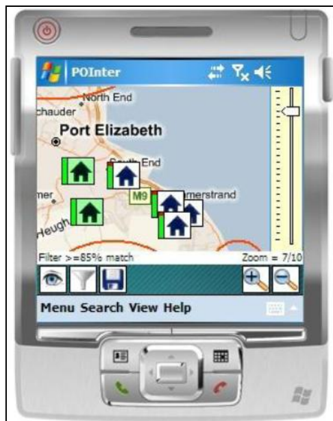
Figure 2.7: POInter supports zooming through the use of step-wise plus or minus icons in the bottom-right-hand corner of the toolbar
