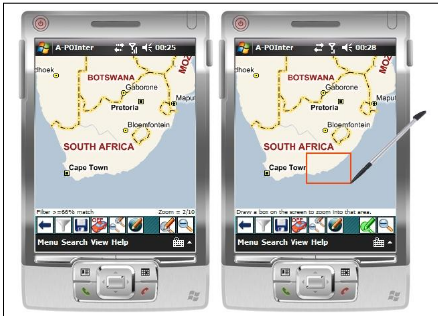
Figure 5.17: Bounding box technique active (left) and drawing a box using the stylus (right)
