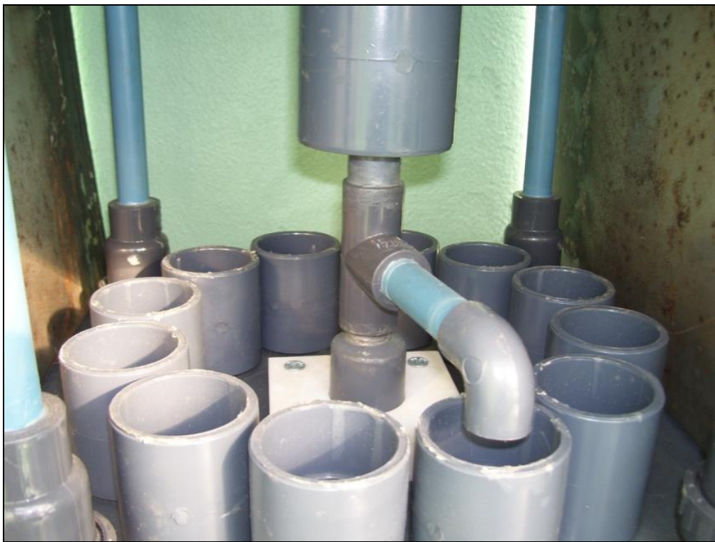
Figure 2: The multiplexer with its rotary arm and the receiving funnels.
