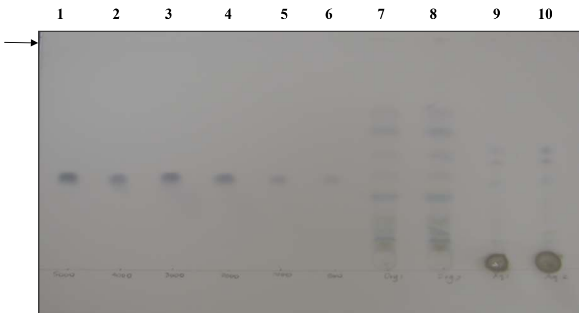
Figure 3.1: A typical TLC chromatogram depicting the identification of the marrubiin content from the OL and AL extracts. Lanes 1-6 have decreasing concentrations of the marrubiin standard (5000, 4000, 3000, 2000, 1000 and 500ng, respectively). Lane 7-8, the OL extract (10mg/ml) and lane 9-10 the AL extract (10mg/ml). Five microlitres of each extract was loaded. The arrow indicates the solvent front.
