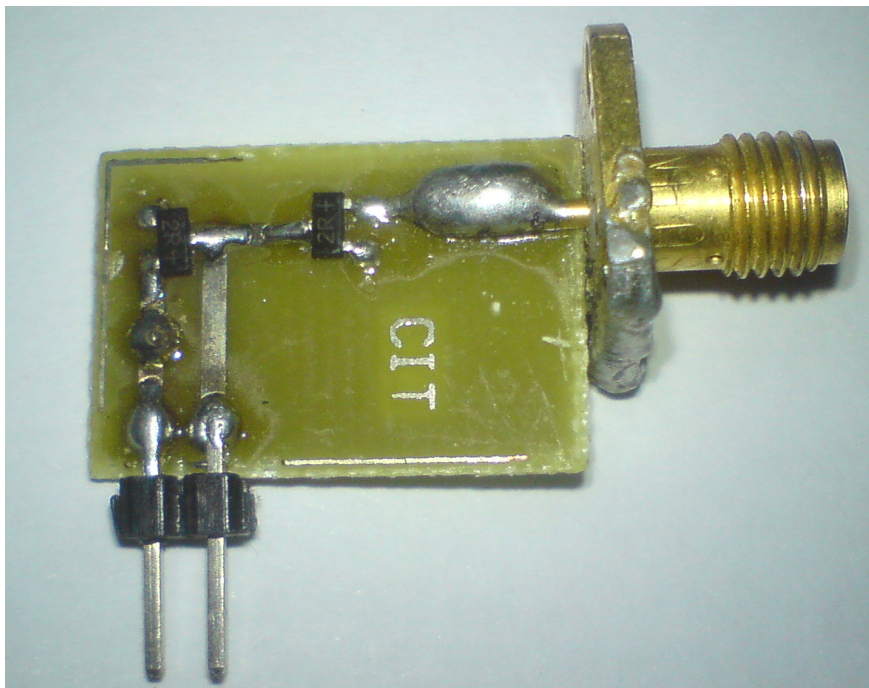
Figure 4. 5: Half wave rectifier with the SMA connector
