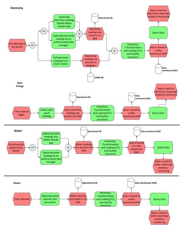
Figure 4.17: To-Be Processes of the Environmental Indicators at NMMU
