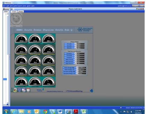
Figure 4.5: NMMU Physics Building's Electricity Usage Dashboard of the JCBMS
