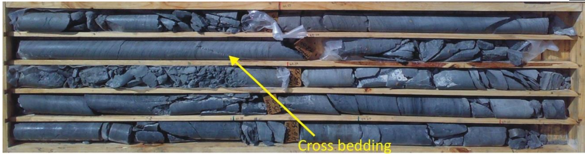
Figure 5.9: Medium dark grey, fine-grained and fractured sandstone of the Goudini Formation observed on borehole NEW24, between 39.56 – 47.16 m below ground level, 1.5 km NNW of Thyspunt. Note the cross-bedding.
