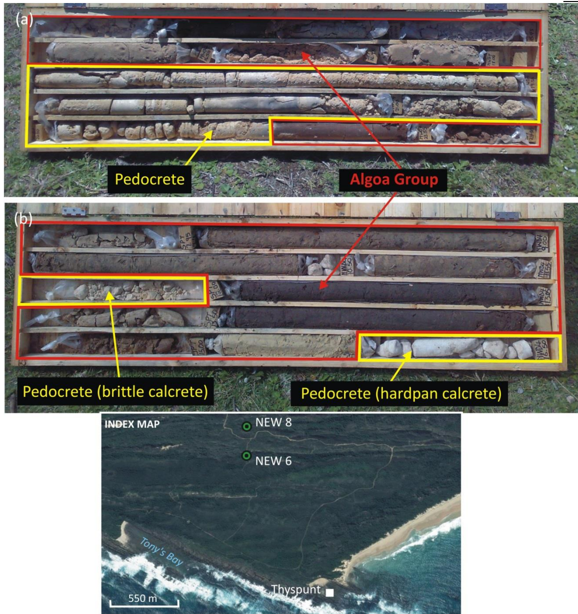
Figure 5.25: (a) A 5.15 m thick pedocrete (calcrete) intercepted in borehole NEW6. The fine-grained pedocretes range from brittle, semi-consolidated, containing cavities to well cemented hardpan calcrete at depths between 18 – 23.15 m below ground surface (33.206 – 28.056 m asl) in borehole NEW6. (b) Pedocrete layers intercepted at depths between 10.45 – 10.50 m (29.844 – 29.794 m asl) and 15.45 – 16.50 m (24.844 – 23.794 m asl) in borehole NEW8.
