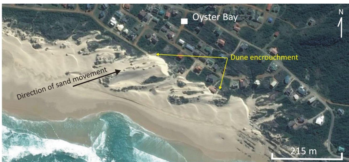
Figure 5.35: Dunes encroaching onto developed land, and holiday home properties in Oyster Bay.
