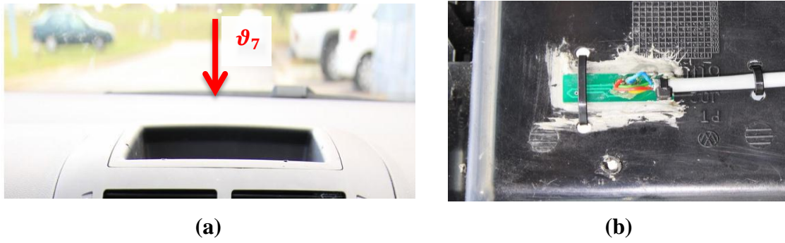
Figure 3-17: Measurement of dashboard temperature; (a) Sensor position, (b) Sensor installation
