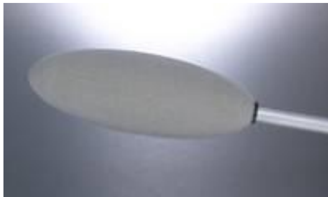
Figure 2-11: Ellipsoid thermal comfort transducer [96]
