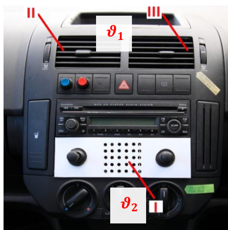
Figure 3-14: Temperature sensor locations
