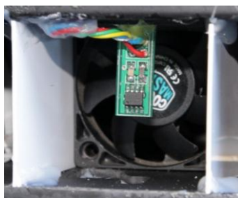
Figure 3-15: Installation of fan-aspirated sensor element
