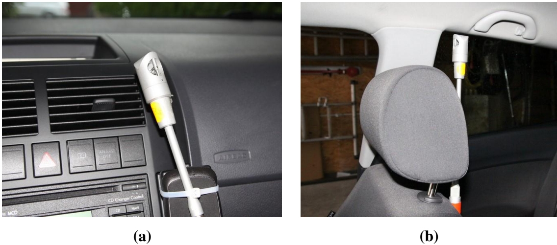
Figure 3-2: Air velocity measurements; (a) Front air outlet, (b) Passenger head
