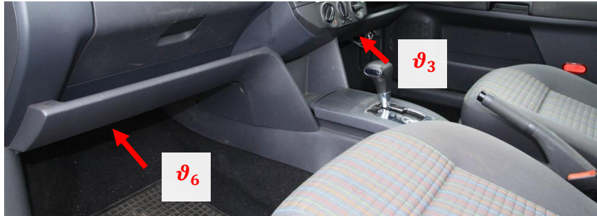
Figure 3-19: Temperature sensor positions at feet level
