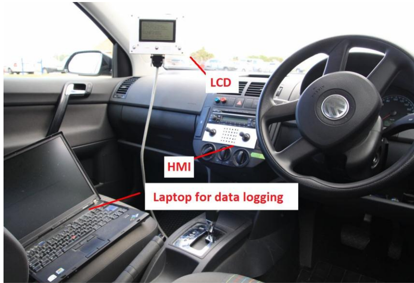
Figure 3-10: HMI and display installation
