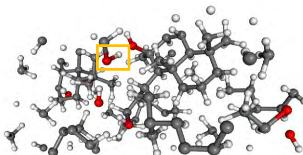
Figure 4.13: Stage two of transfer with the hydrogen-oxygen bond of the donor hydroxyl group (orange rectangle) extending towards the acceptor.
