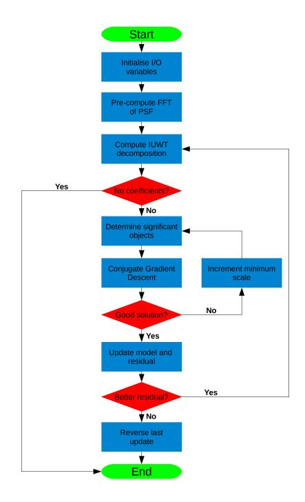
FIGURE 3.1: Simplified flowchart which details the operation of PyMORESANE.
