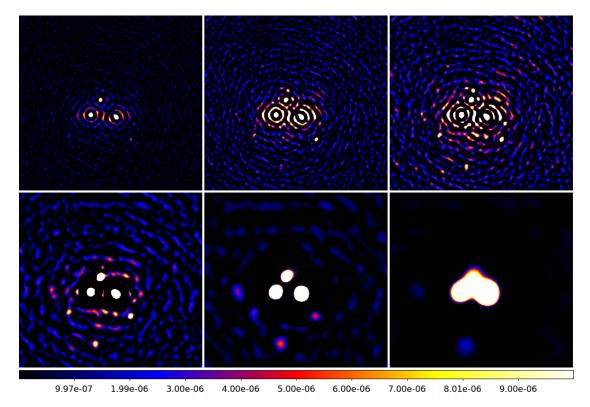
FIGURE 2.4: Six plane IUWT second-generation decomposition of synthetic data. The images are in order of ascending scale from top left to bottom right.
