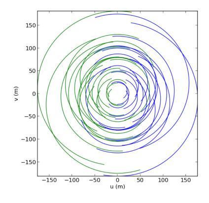
FIGURE 2.1: Coverage of the uv-plane for a simulated KAT7 observation.
