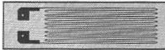
Figure 23: A wire strain gauge bonded on elastic backing (Fraden, 2004, p. 326)
