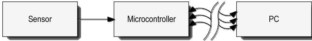
Figure 24: Sending the sensor data wirelessly to the PC
