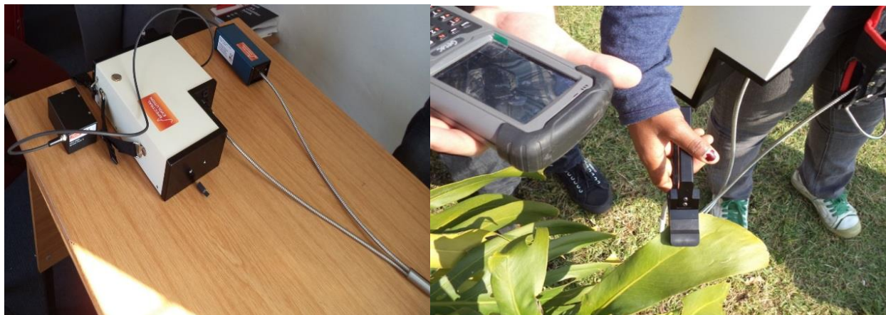
Plate 4.2: The Spectral Evolution Spectroradiometer PSR3500 series
