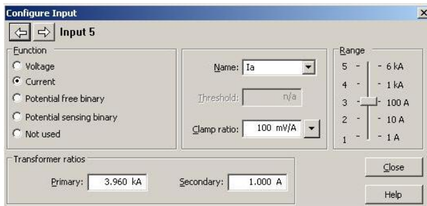
Figure 10: Clamp on CT setup within OMICRON EnerLyzer
