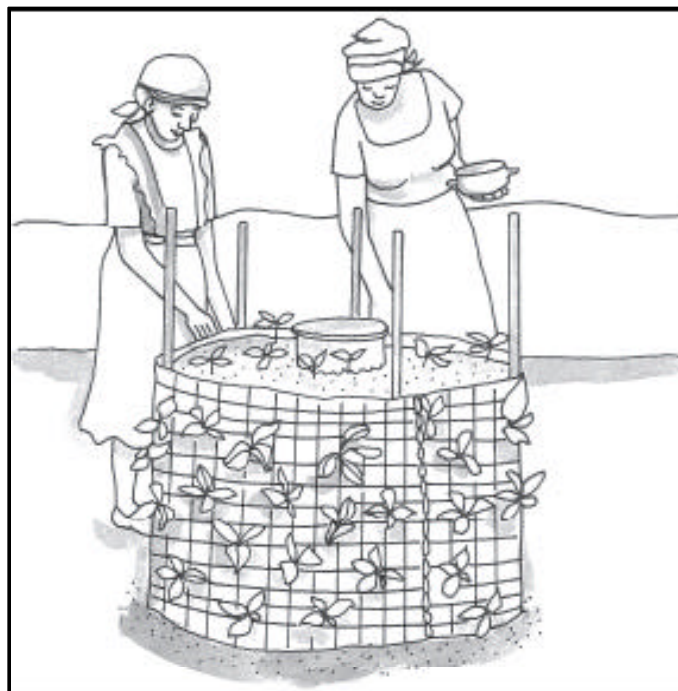
Figure 5.2: Grey water soak-away of the tower garden type (Crosby, 2004).
