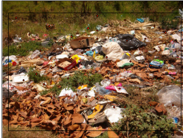
Figure 3.3: A grid consisting of randomly placed dots was used to determine the types and sources of solid waste.
