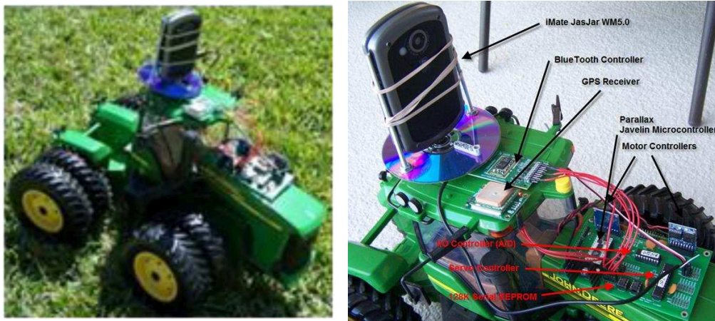
Figure 3.9: NiVek J.D. (left) and its Components (right)
