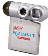
Figure 2.6: A FlyCAM Camera that Connects to the CF Slot
