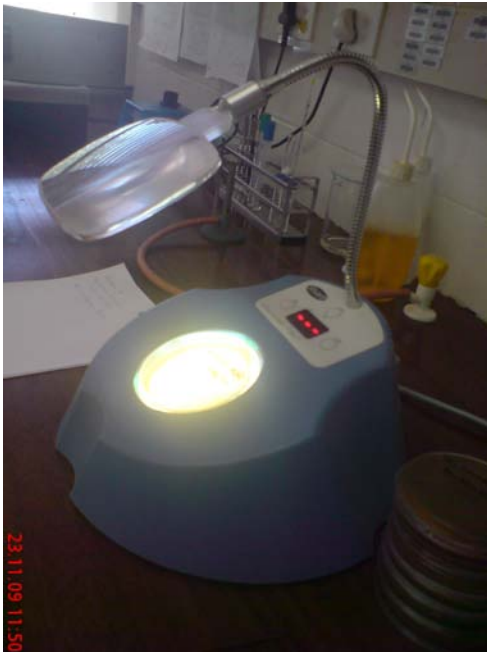
Fig 5.25 Colony counter used to count the revertant colonies on the Ames test
