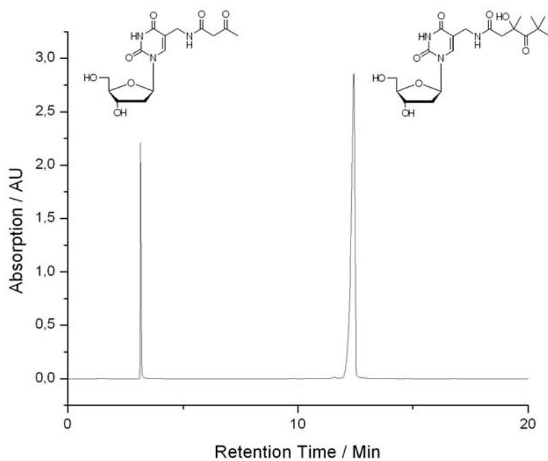
Figure B.2 HPLC chromatogram of 3 after irradiation. Ketone 7 is detected as a product at short retention time.
