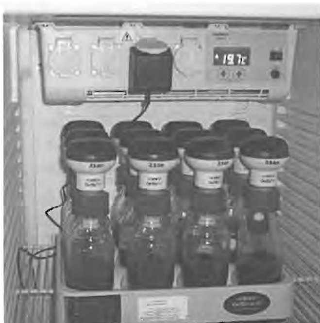
Figure 6.1a: The OxiTop system on the stirring pad
