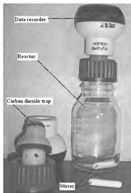
Figure 6.1b: Components of the OxiTop reactor
