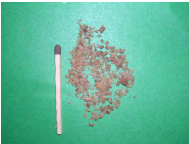
Figure 4.3 Yeast cells immobilized on the surface of silica gel particles. The match provides a size scale (1.2× magnification).
