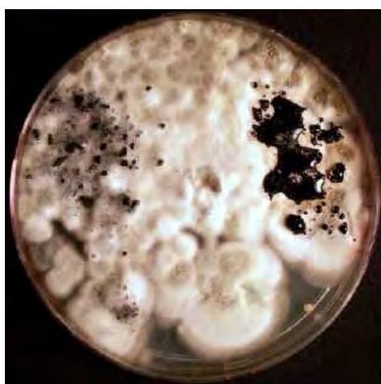
Figure 2-3 Gutation droplet formation on 4.69 N HNO 3 treated bituminous hard coal (right) after 3 days contact with a fully grown culture of ECCN 84. No change yet was observed in the untreated bituminous hard coal (left).
