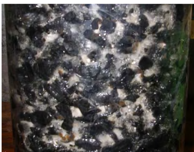
Figure 6-4 Biofilm formation on the surface of bituminous hard coal in the fixed-bed perfusion column bioreactor that was perfused with a low molecular weight organics carbon supplement.
