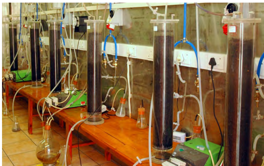
Figure 6-3 Experimental set up of the fixed-bed perfusion column bioreactors in a constant environmental laboratory held at 28 °C.
