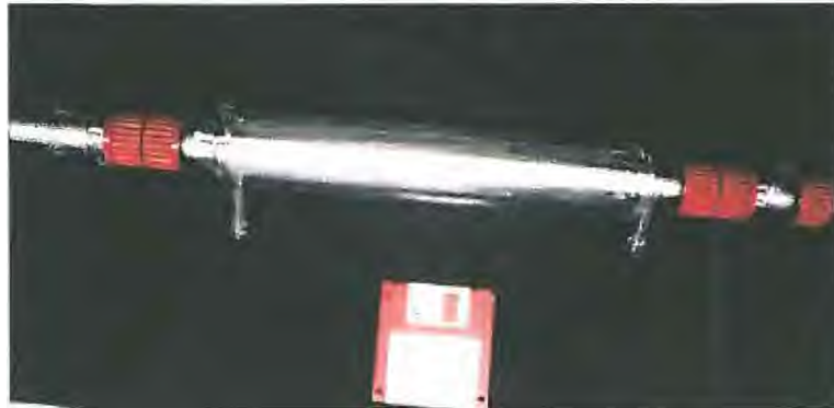
Fig 5.1: Cylindrical axial flow fibre bundle membrane bioreactor.
