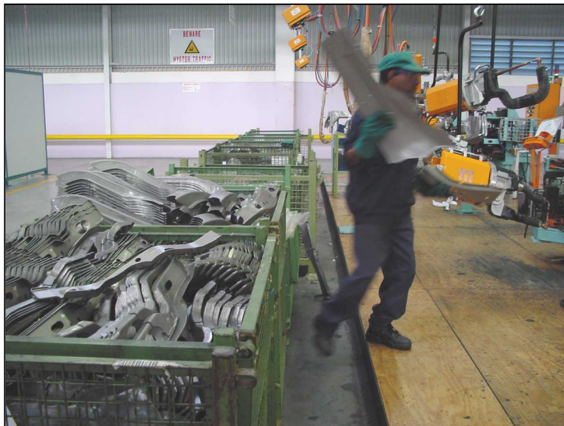
Figure 1: A Bodyshop operator is required to lift and carry a body panel from an industrial storage bin in a South African automotive industry.
