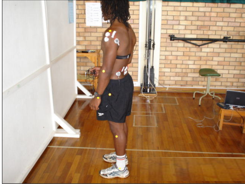
Figure 11: Participant setup and electrode placement on the medial deltoid (left and right) and erector spinae (left and right). (Task 1: PTT)
