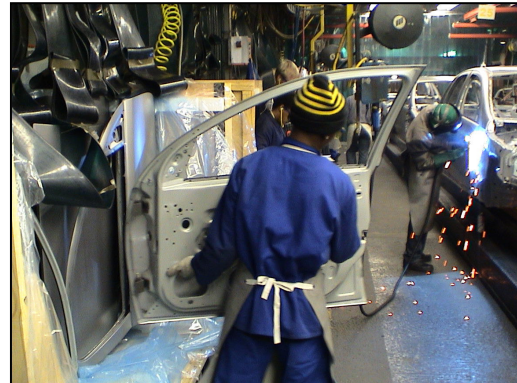
b Twists and carries door from the crate on the Closure Line
