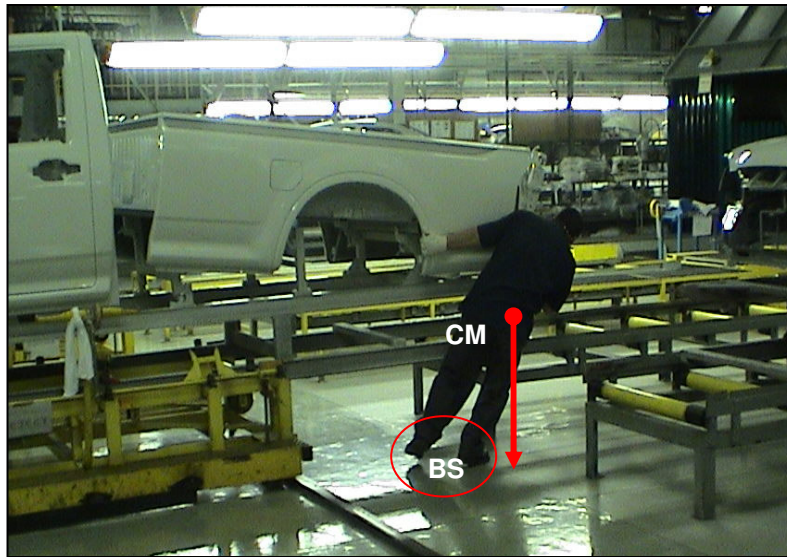
Figure 13: Working posture showing pulling with centre of mass (CM) outside the base of support (BS) in the Paintshop at the GM Plant.
