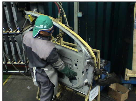
d Places the door on the hoisting jig
