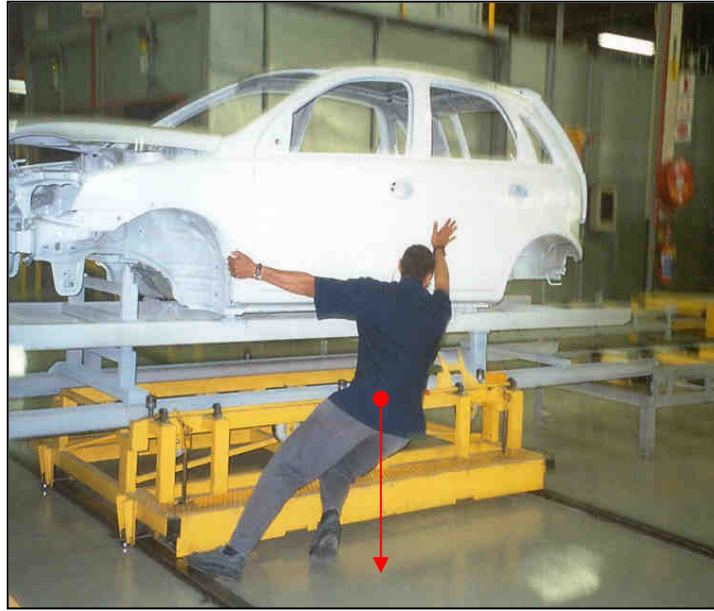
Figure 3: The pulling of a vehicle frame on a trolley platform.
