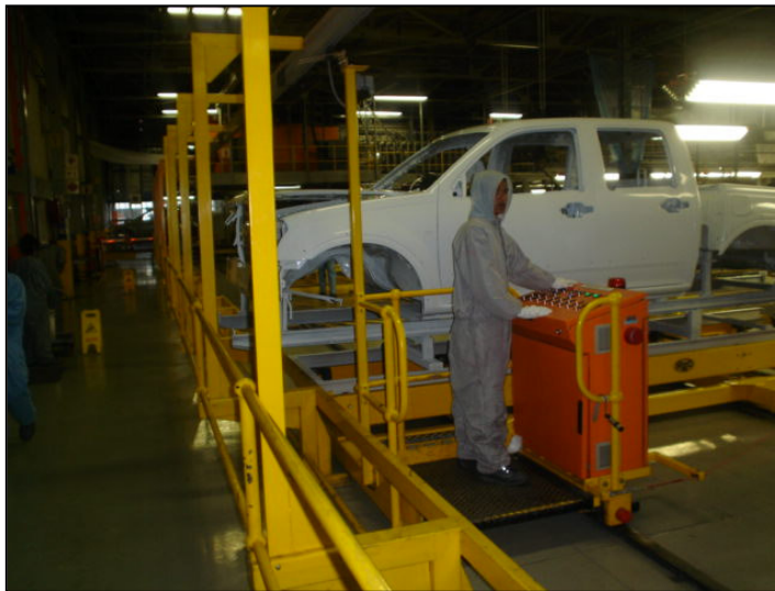
Figure 42: Automated transfer trolley used in the Paintshop post-intervention.
