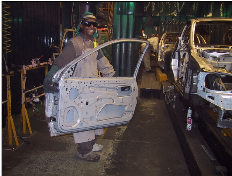
Figure 2: A Bodyshop operator manually lifts a car door on the closure line.
