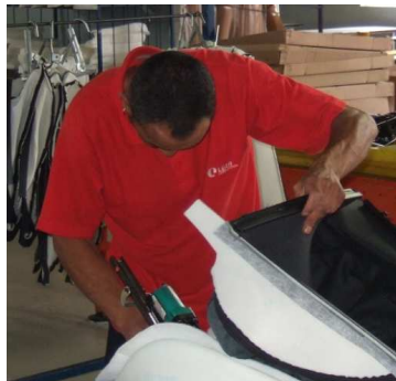
Screwing during seat manufacturing and in assembly line
