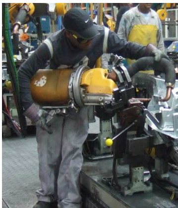
Welding tasks in body shop
