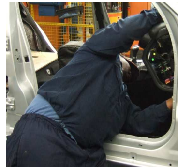
Clipping dashboard in assembly line
