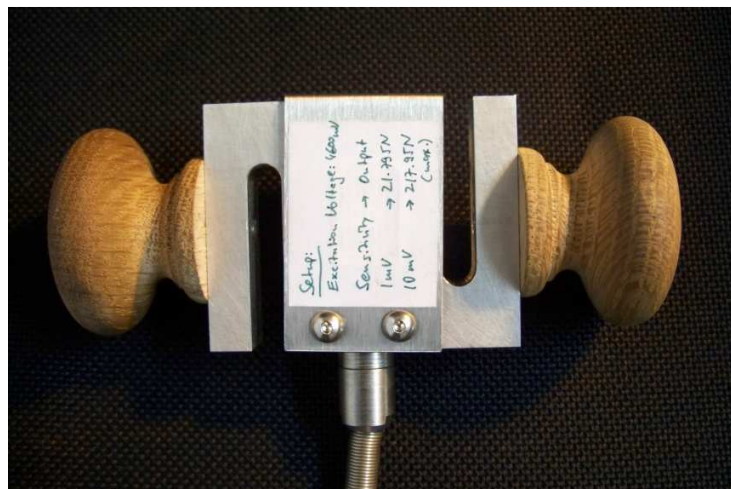
Figure 2.6: Load cell with handles
