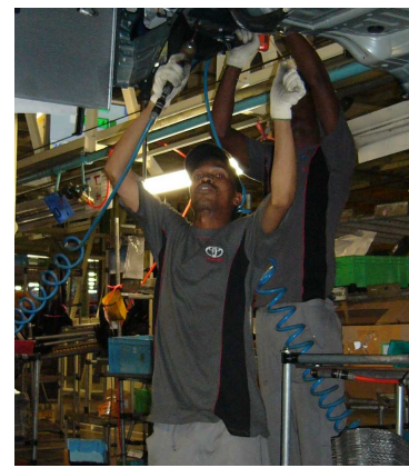
Screwing overhead in assembly line
