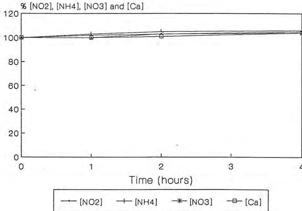
**Figure 29:** Percentage changes in nitrite, total ammonia, nitrate and calcium concentrations during the one-hour oxygen trials in the experimental system B.
