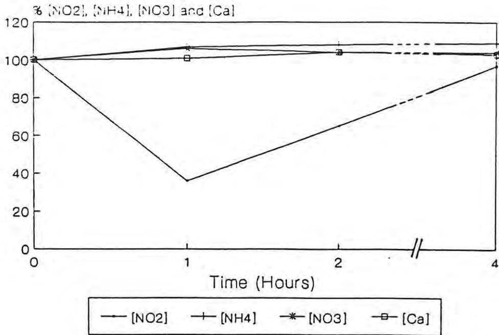
**Figure 21a:** Percentage changes in nitrite, total ammonia, nitrate and calcium concentrations during and after the one-hour, low-dose ozone trials in the experimental system B.
