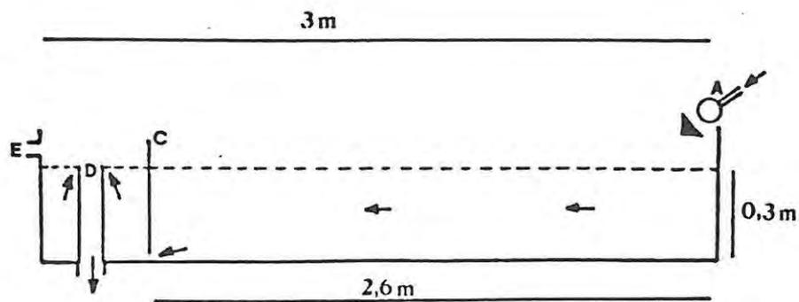
Figure 2b: Cross-section of culture tank with annotation as for Fig. 2a. Arrows indicate water flow.
