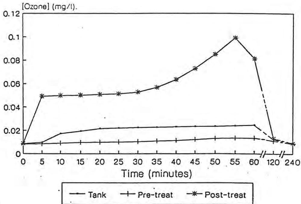
**Figure 20:** Ozone concentrations measured in the culture tanks, and immediately pre- and post-treatment in the contact chamber, during and after the one-hour, low-dose trials.
