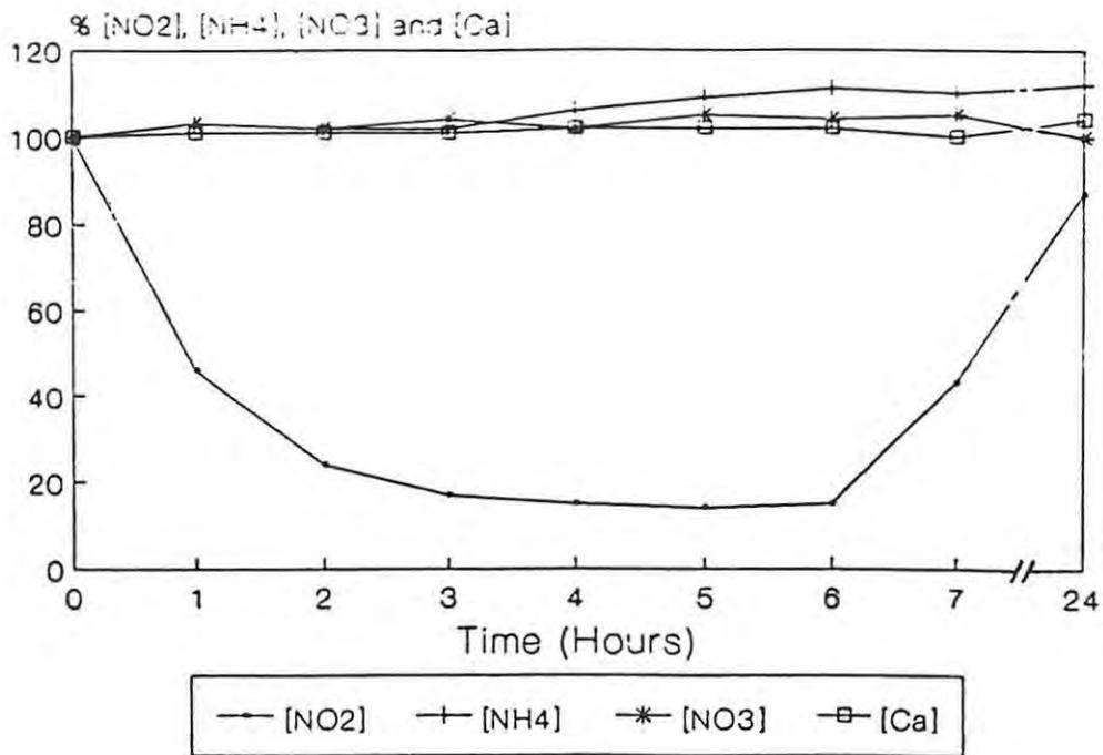
**Figure 24a:** Percentage changes in nitrite, total ammonia, nitrate and calcium concentrations during the six-hour, low-dose trials in the experimental system B.
