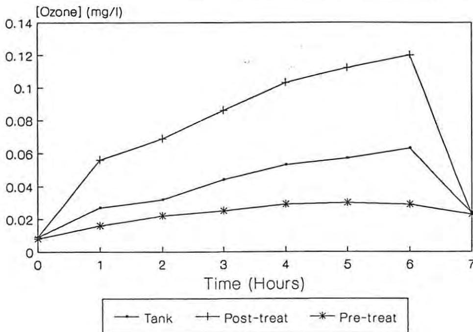
**Figure 23:** Ozone concentrations measured in the culture tanks, and immediately pre- and post-treatment in the contact chamber, during and after the six-hour, low-dose trials.
