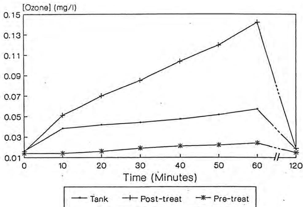
Figure 26: Ozone concentrations measured in the culture tanks, and immediately pre- and post-treatment in the contact chamber, during and after the one-hour, high-dose trials.
