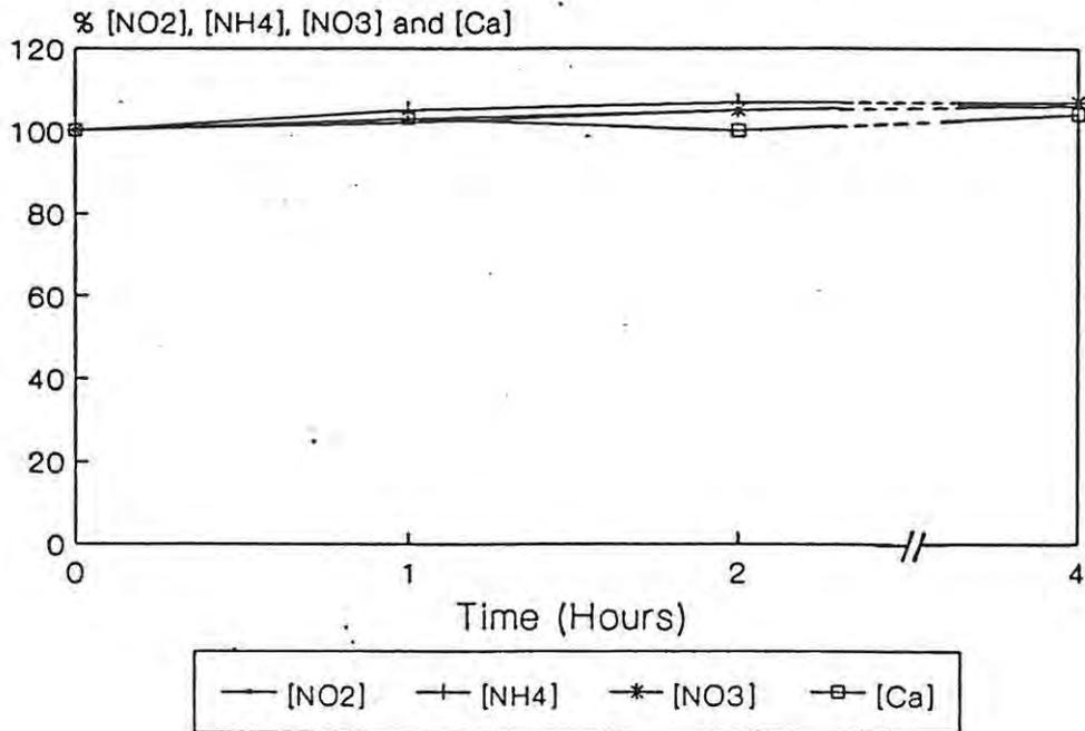
**Figure 21b:** Percentage changes in nitrite, total ammonia, nitrate and calcium during and after the one-hour, low-dose trials in the control system A.
