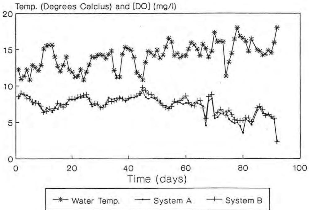
**Figure 16:** Water temperature, and changes in dissolved oxygen (DO) concentrations in systems A and B during the study.
