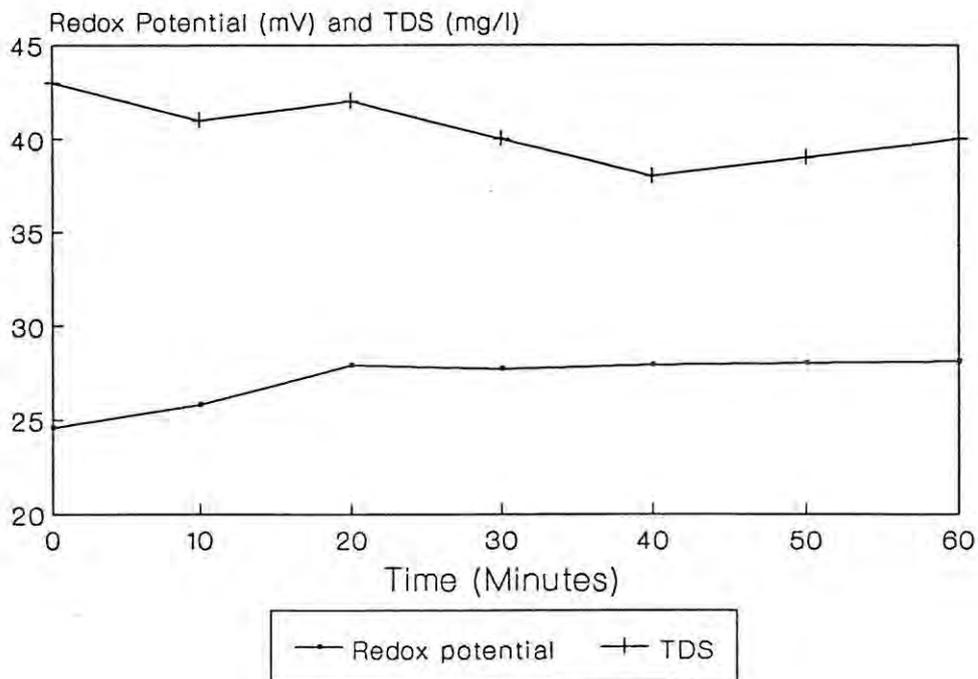
**Figure 22:** Changes in redox potential and total dissolved solids (TDS) during the one-hour, low-dose trials, in the experimental system B.
