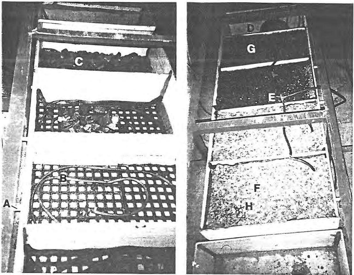
Figure 4a: Photographs of the biological filter, with A) sludge draw-off pipe, B) false bottom with sub-gravel aeration pipe attached, C) large 50 mm gravel, D) pumping chamber, E) sub-gravel aeration attached to air supply, F) 19 mm gravel, G) 10 mm gravel H) shade-cloth between gravel layers.
