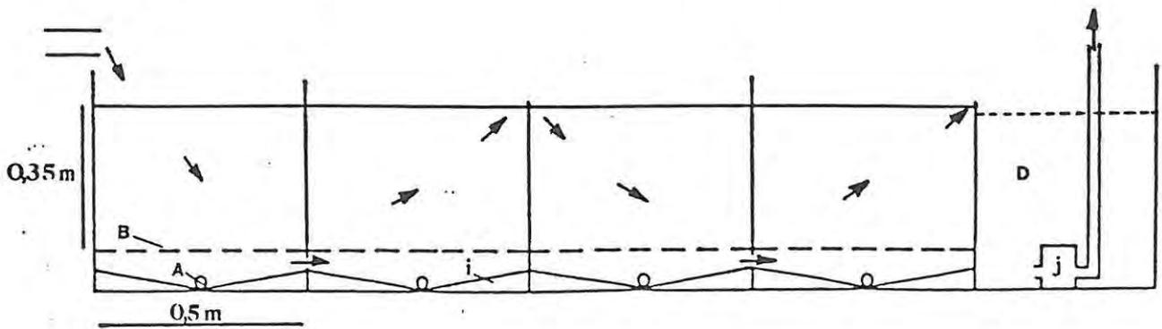
Figure 4b: Cross-section of biological filter, with annotation as for Fig. 4a. (i = V-shaped bottom, j = pump). Arrows indicate water flow.
