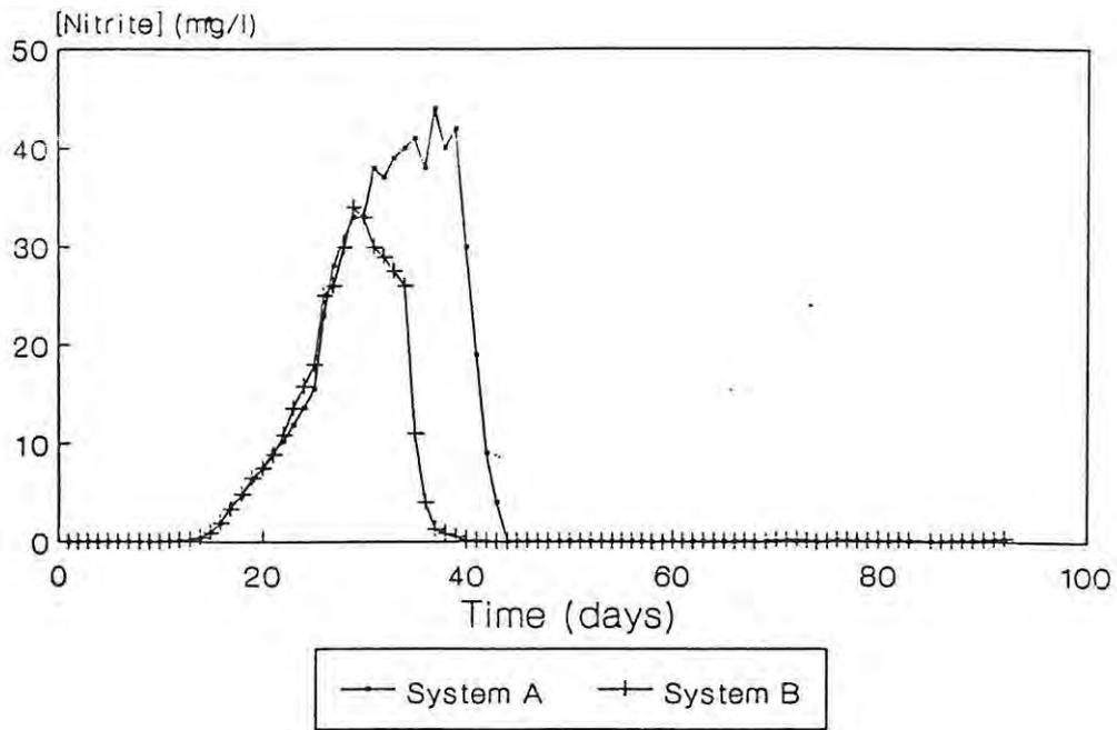
**Figure 10a:** Changes in nitrite ( $\text{NO}_2\text{-N}$ ) concentrations in systems A and B during the study.
