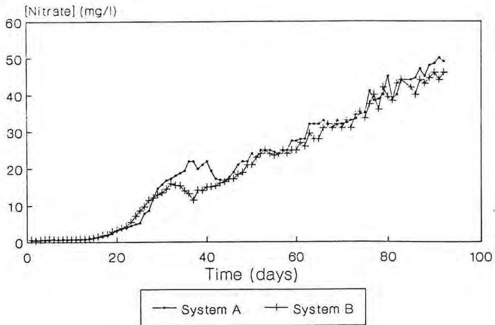
**Figure 11:** Changes in nitrate ( $\text{NO}_3\text{-N}$ ) concentrations in systems A and B during the study.
