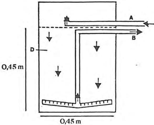
Figure 5b: Cross-section of activated carbon filter, with arrows indicating direction of water flow (D = activated carbon).
