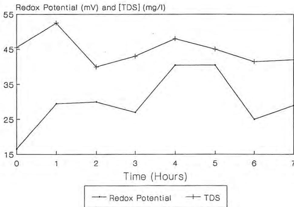
**Figure 25:** Changes in redox potential and total dissolved solids (TDS) during the six-hour, low-dose trials in the experimental system B.
