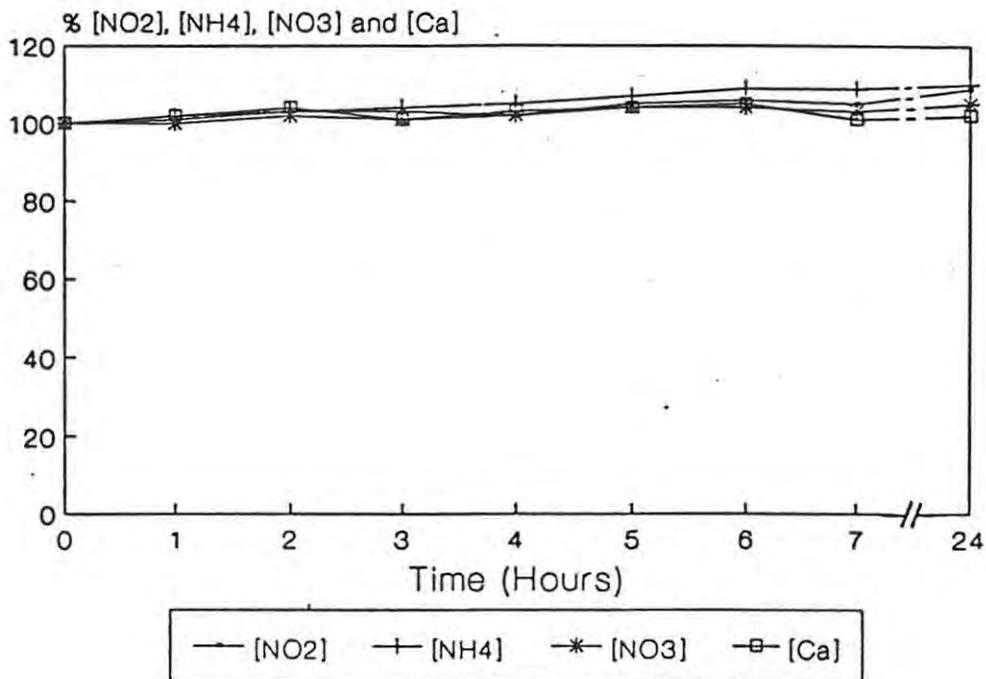
**Figure 24b:** Percentage changes in nitrite, total ammonia, nitrate and calcium concentrations during the six-hour, low-dose trials in the control system A.
