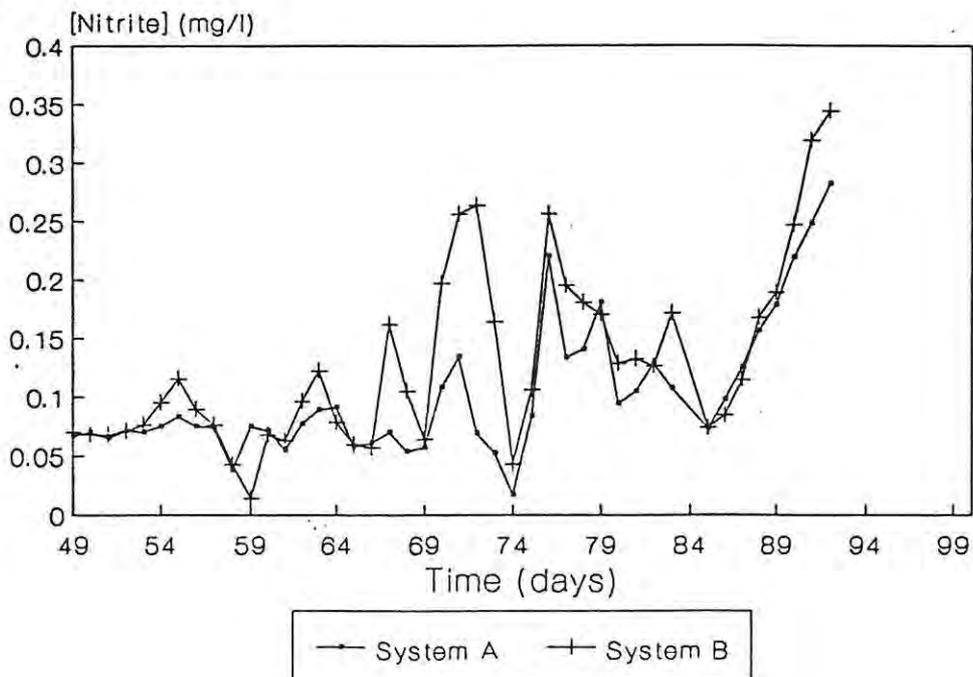
**Figure 10b:** Changes in nitrite ( $\text{NO}_2\text{-N}$ ) concentrations in systems A and B from days 49 - 92 of the study.
