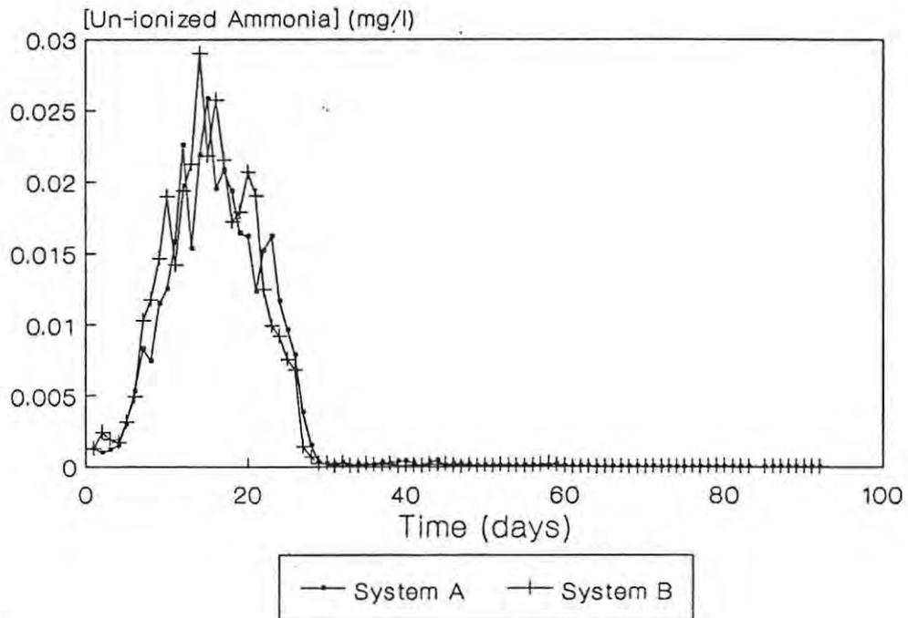
**Figure 9:** Changes in un-ionised ammonia ( $\text{NH}_3$ ) concentrations in systems A and B during the study.
