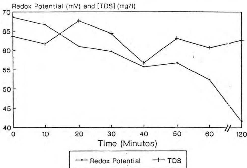
Figure 28: Changes in redox potential and total dissolved solids (TDS) during the one-hour, high-dose trials in the experimental system B.
