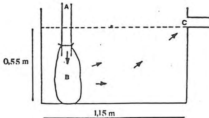
Figure 3b: Cross-section of sedimentation tank with annotation as for Fig. 3a. Arrows indicate water flow.
