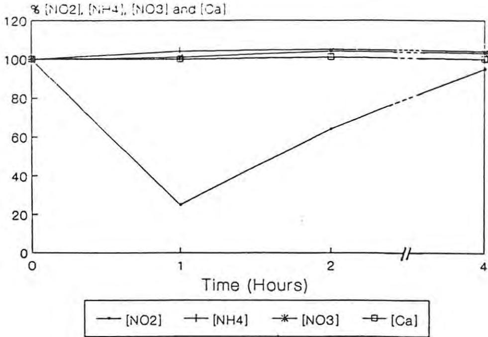
**Figure 27a:** Percentage changes in nitrite, total ammonia, nitrate and calcium concentrations during and after the one-hour, high-dose trials in the experimental system B.
