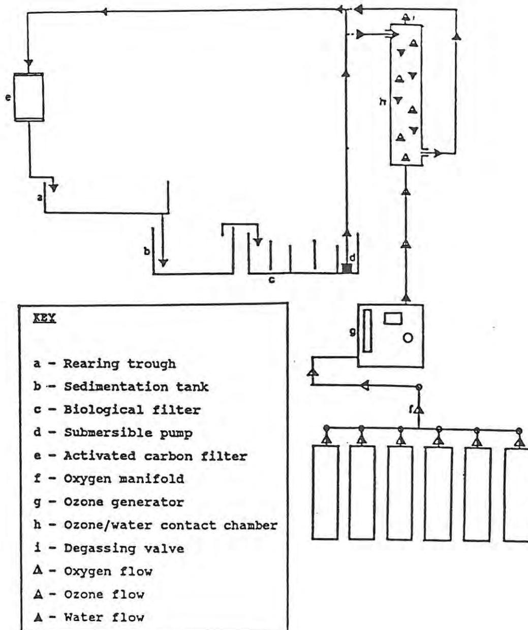
Figure 1: Diagram illustrating the experimental system (not to scale). Components f, g, h and i incorporated only in System B.
