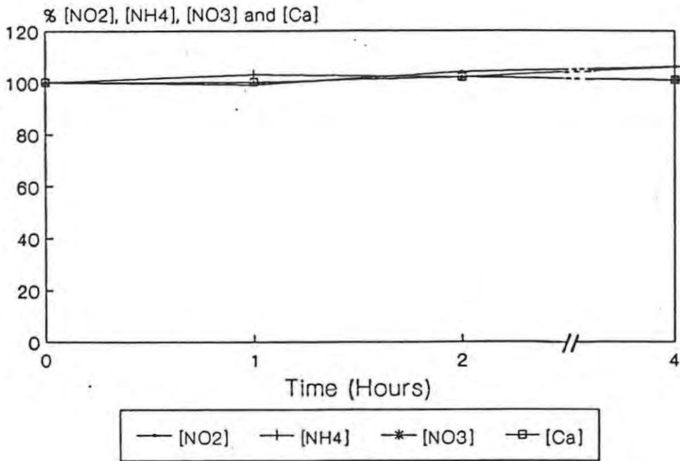
**Figure 27b:** Percentage changes in nitrite, total ammonia, nitrate and calcium concentrations during and after the one-hour, high-dose trials in the control system A.
