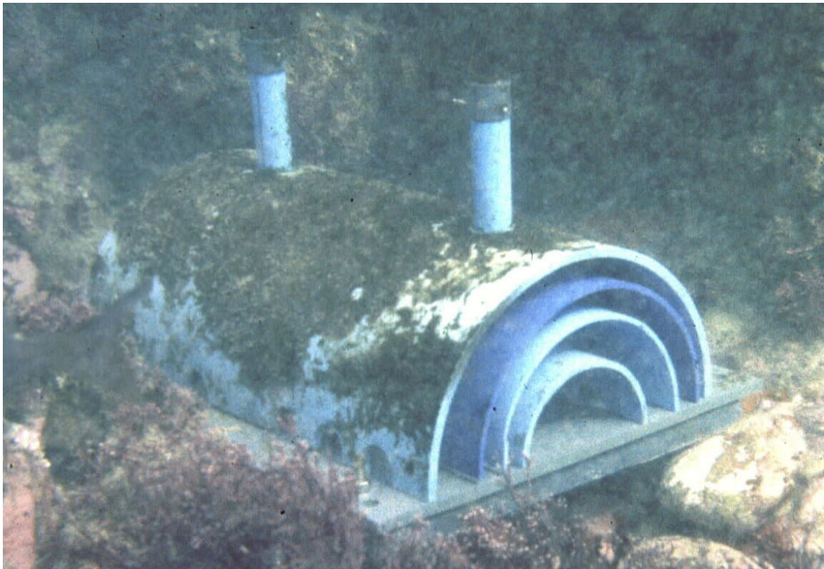
Figure 3.3 Release module in place on the seafloor. Note the ballast weight attached to the underside.
