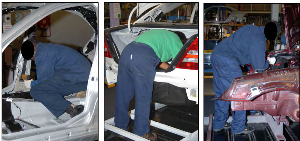
Figure 1: Examples of assembly work in the automotive industry involving the interaction between manipulative tasks and awkward working postures.
