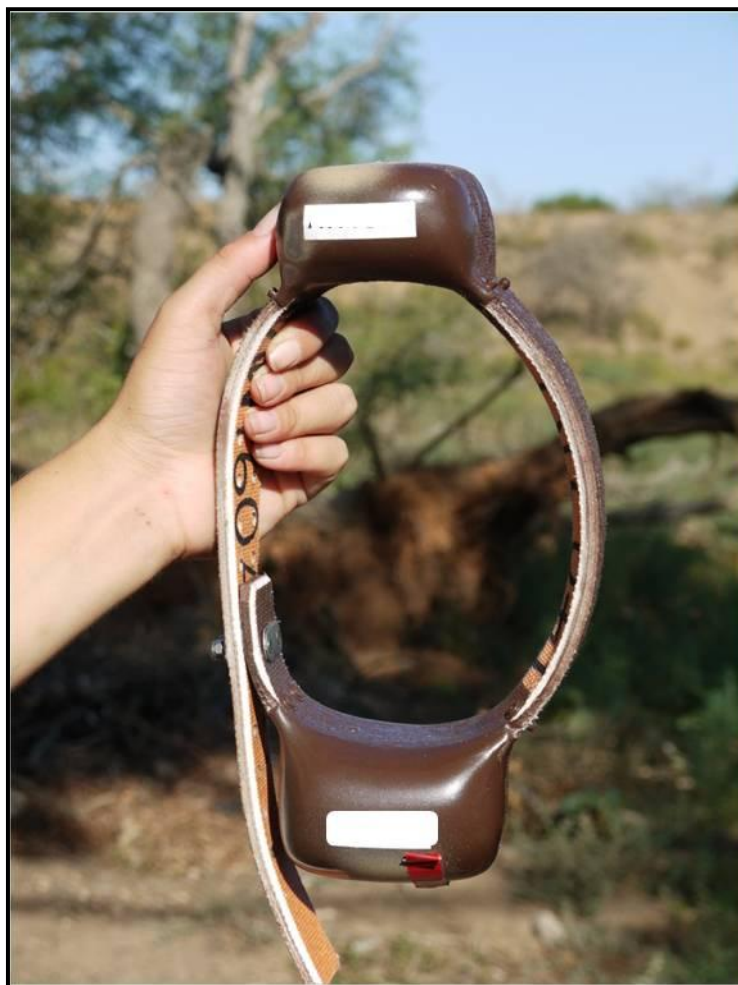
Figure 4.4: GPS/VHF collar; VHF is the larger unit on the underside of the collar and the GPS unit is smaller and points upwards towards satellites.
