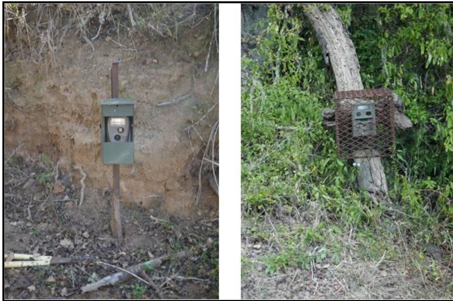
Figure 3.4: The use of different attachment points for camera placement, dependent on the surrounding area and vegetation.
