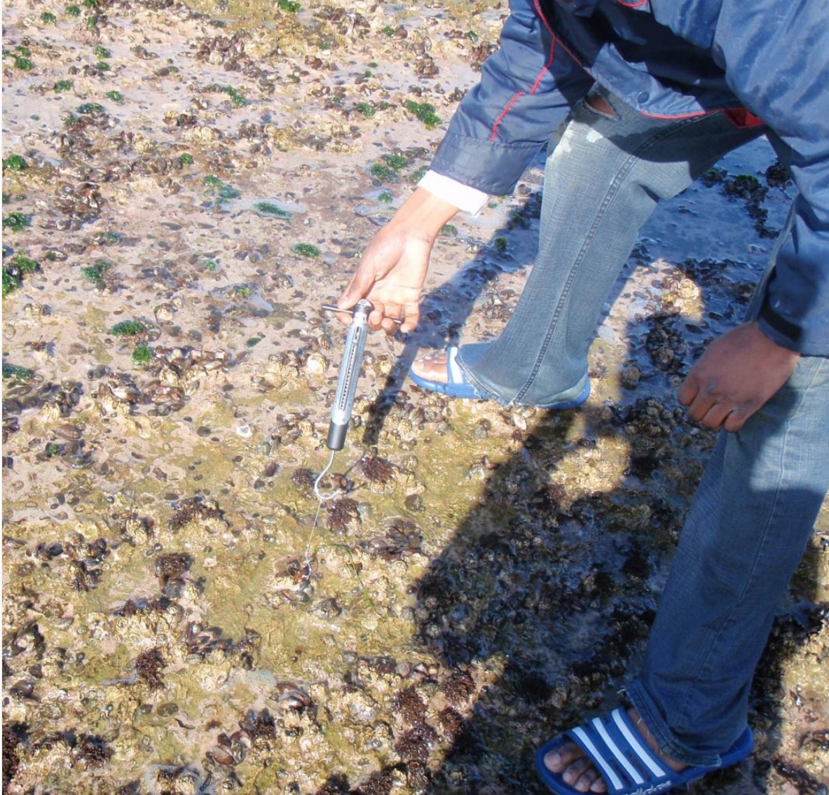
Figure 2.3. Measurement of tenacity/ attachment strength of mussel using a spring balance.
