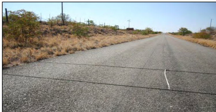
Figure 4.10: A photograph demonstrating the placement of the two traffic tubes (150 cm apart) on the paved road with a tape measure at the centre point to ensure accurate placing of the figure-8 grip.
