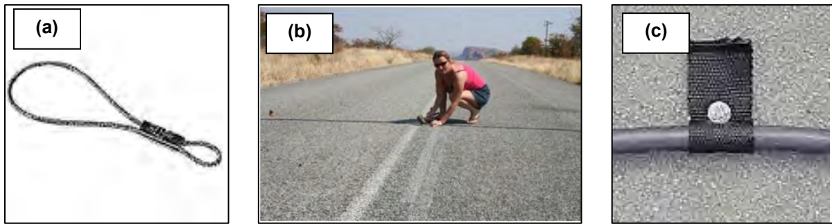
Figure 4.10: Photographs demonstrating the attachment of the road traffic tube to the paved road showing (a) the detail of the figure-8 grip (PicoCount 2500 Traffic Counter Manual 2009), (b) the attachment of the traffic tube to the paved road surface using a 150 mm masonry nail to secure the figure-8 grip and, (c) the detail of the attached traffic tube showing duct tape and 150 mm masonry nail to secure it in place.
