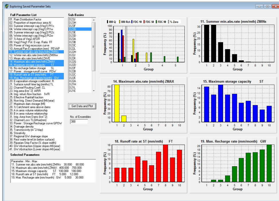
Figure 3.3 Illustration of the tool designed to help with determining appropriate parameter bounds.
