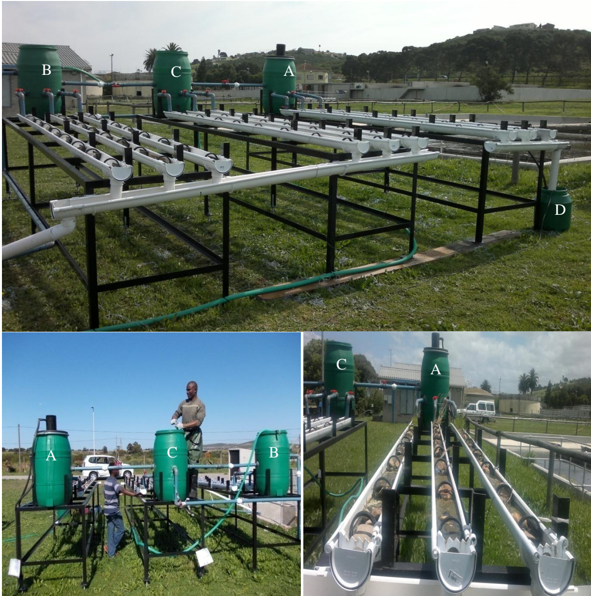
Figure 7.3: The full experimental set-up at the beginning of the experiment (top); the experimental view from behind the upstream of the stream channel (bottom left), and the control streams after 90 days (bottom right). Tanks: A (de-chlorinated tap water), B (100% treated effluent), C (50% treated effluent) and D (50-litre tank with a Pedrollo top 2 pump for recirculation of dechlorinated tap water).
