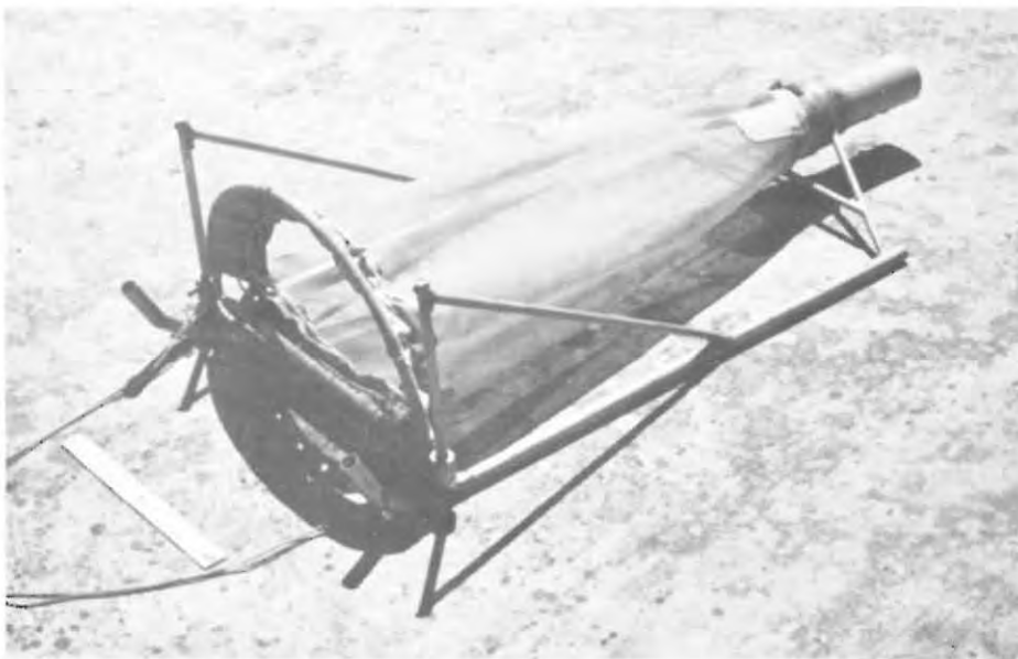
Fig. 19 D-net used to trawl immediately above the substratum.
