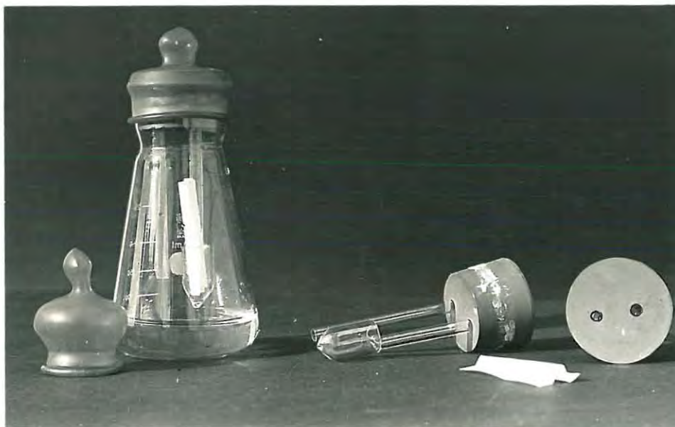
Fig. 7: The 250 ml incubation flasks used in the uptake of acetate and glucose experiments, showing the folded filter paper for the collection of ^{14}\text{CO}_2 , the filter holder and the glass tubing in the rubber bung for the injection of acid through the bottle teat.
