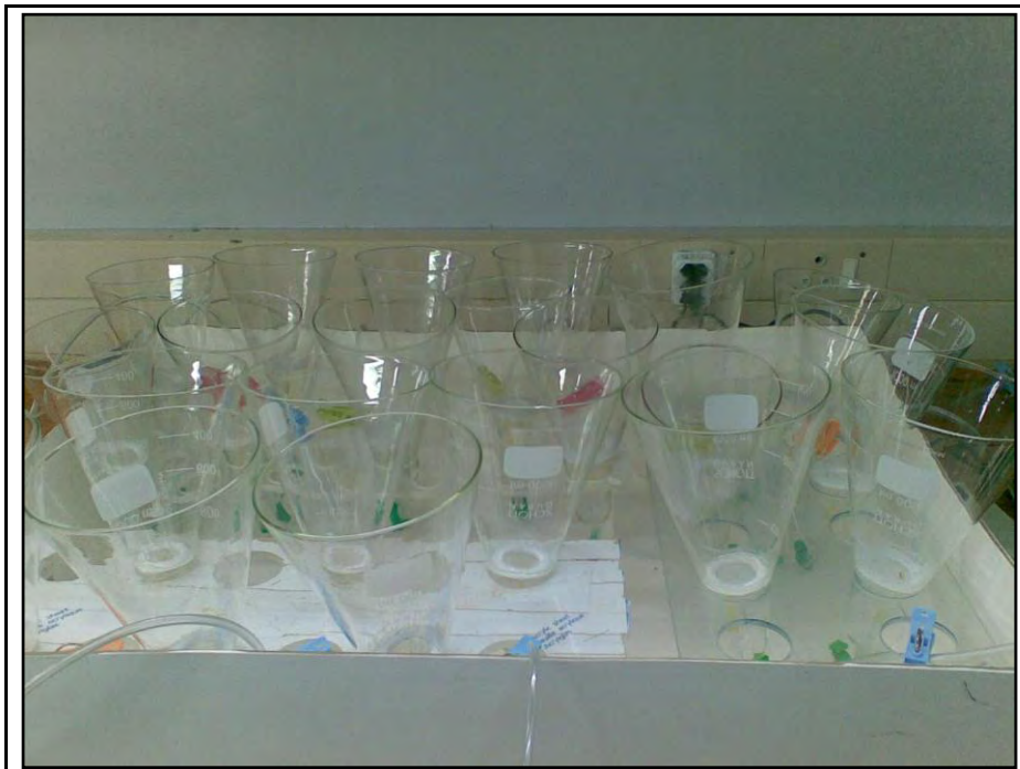
Figure 2.4: Experimental brood chambers for the simulation of C. nilotica brood pouch used for embryo development toxicity tests
