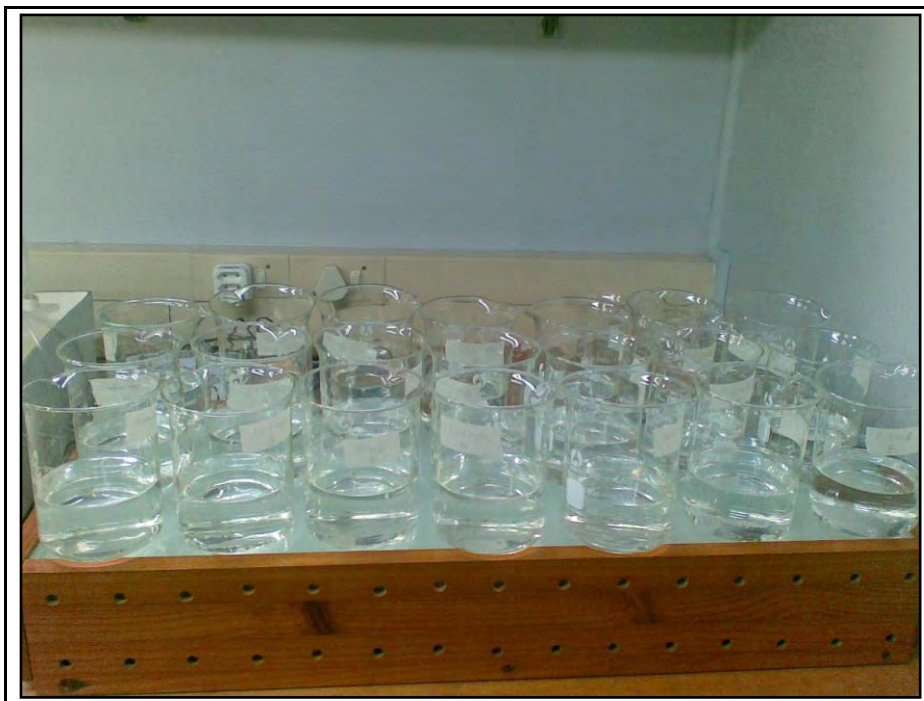
Figure 2.2: Test chambers (600-mL beakers) used for short-term toxicity tests
