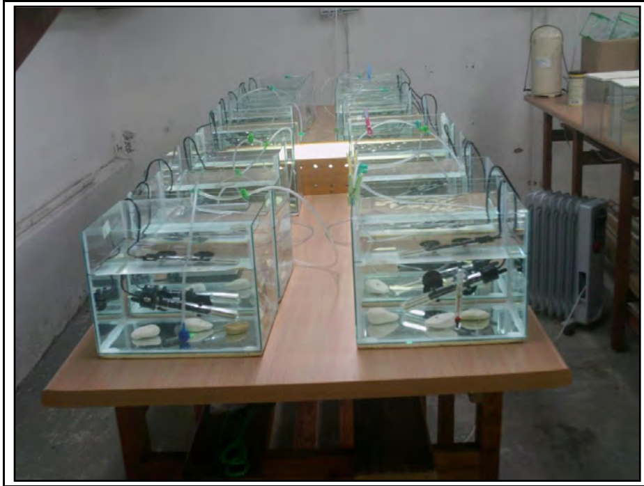
Figure 2.3: Glass tank aquaria (20-L) filled with dechlorinated tap water and supplied with aerators, thermostat heaters, thermometers and water circulation pumps used for long-term toxicity tests
