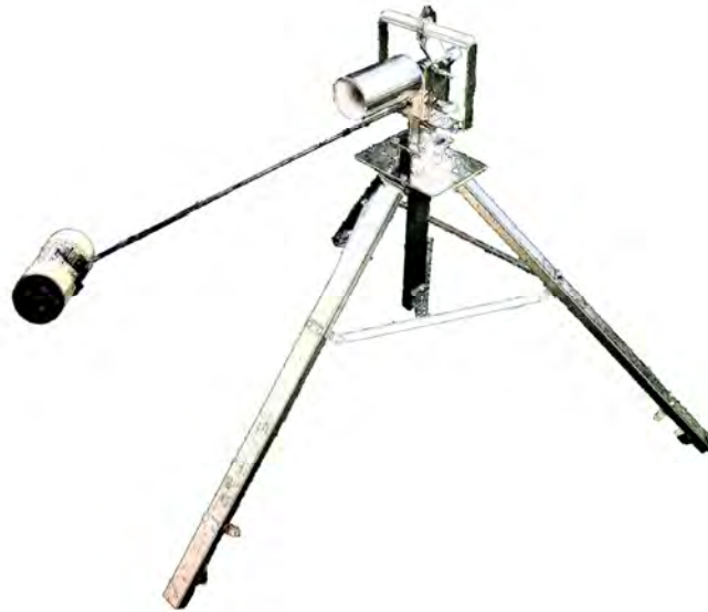
Figure 3.1: Drawing of the tripod used to hold the remote video camera for the remote underwater video (RUV) and baited RUV stations. The bait-arm, holding the PVC bait container is attached. The cable and rope, which clip to the top of the tripod are not shown here.
