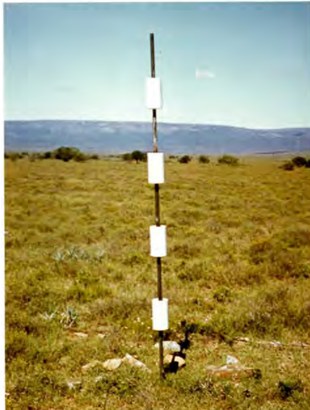
Fig. 47. Set of four sticky cylindrical impact traps used to monitor the vertical distribution (0,5 to 2,0 m) of wind dispersed D.austrinus crawlers.
