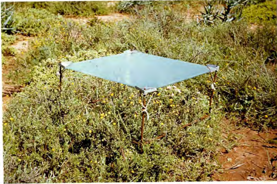
Fig. 45. Horizontal sticky impact trap used to monitor the dispersal of D.austrinus crawlers in the field.
