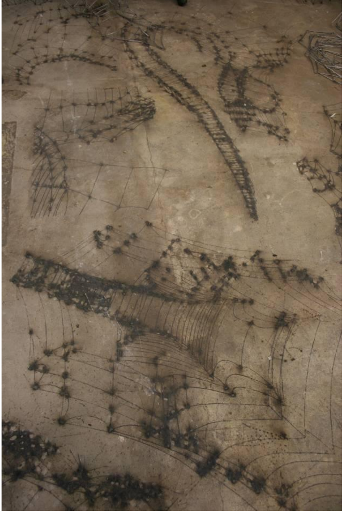
Figure 23. The trace of the burn marks left after welding.
