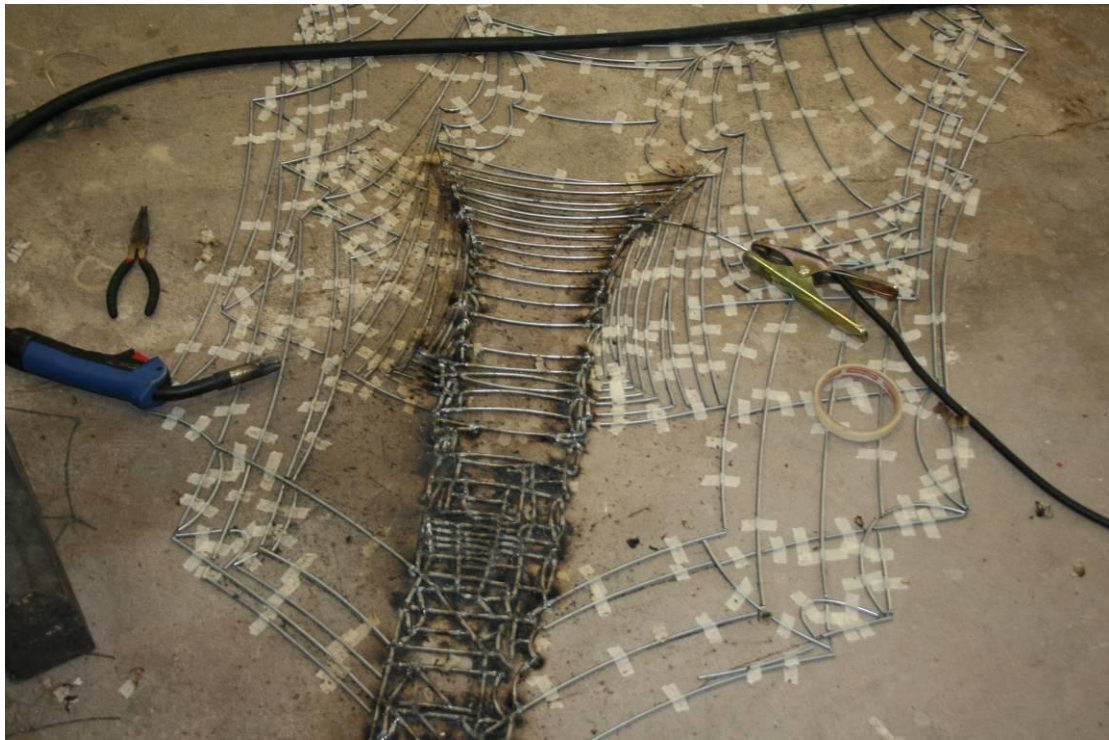
Figures 8.6 – 8.7. Welding the wire together.
