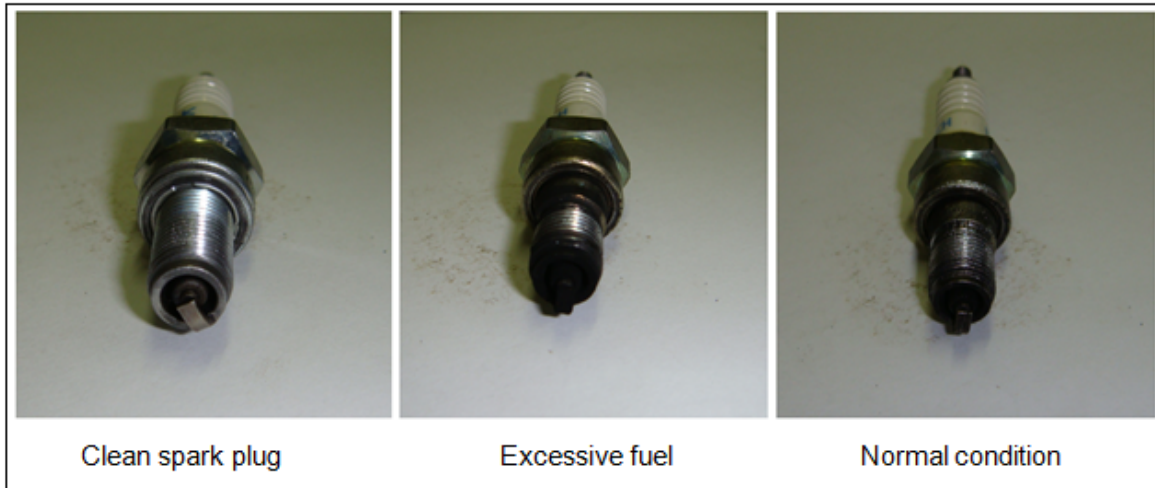
Figure 4.4 Spark plug analysis
